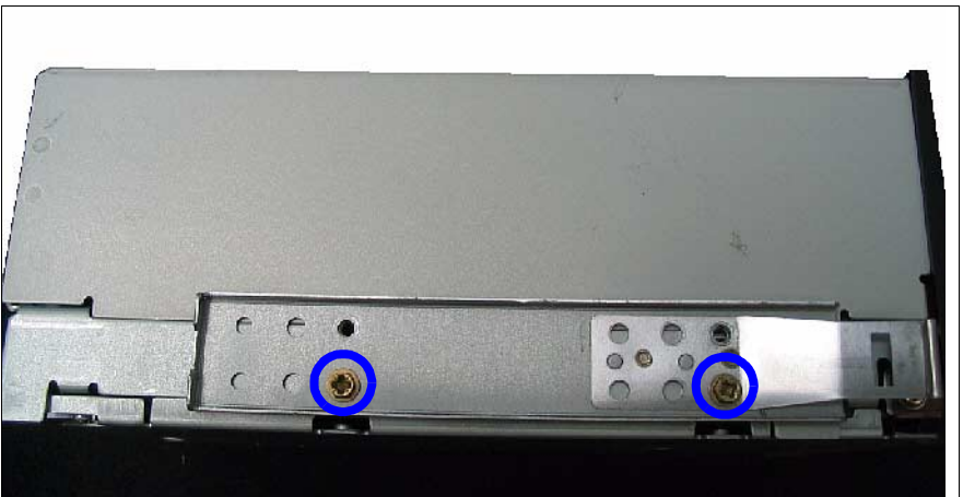
Figure 18: Attaching the EasyClick rails - magnetic tape drive LTO Ultrium 2FH
